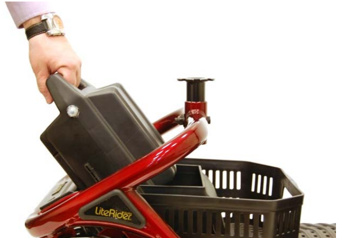
Figure 21. Battery Pack Installation
