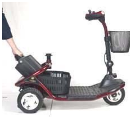
Figure 14. Removing the Battery Pack
