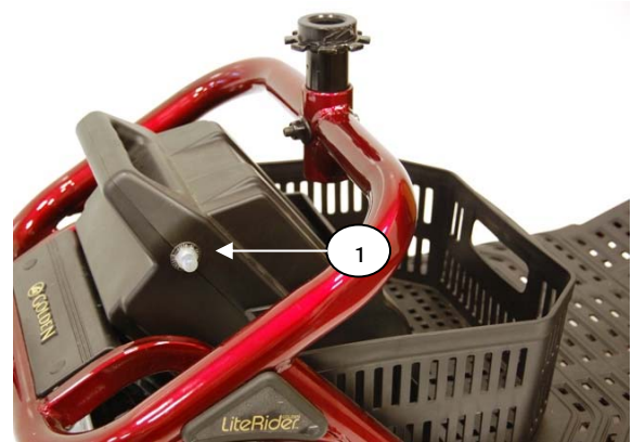
Figure 27. Main Circuit Breaker
