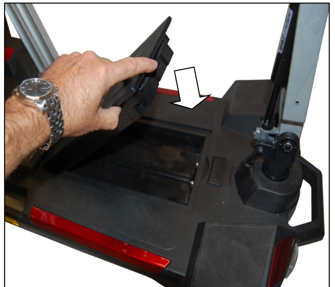
Figure 20. Installing Battery Pack
