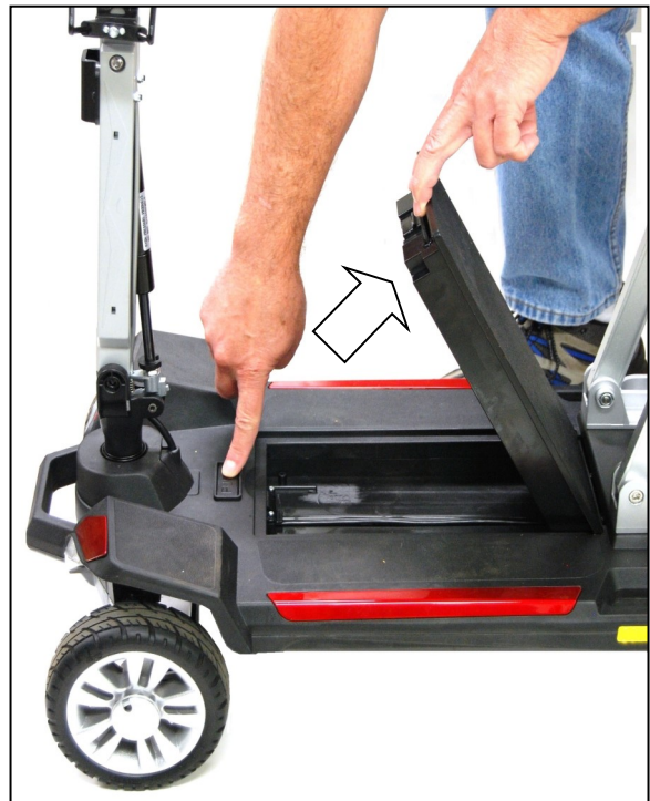
Figure 13. Removing Battery Pack
