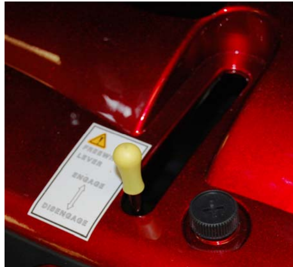
FIGURE 12. FREEWHEEL LEVER (DISENGAGED)
