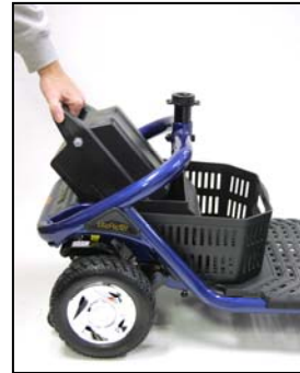
Figure 14. Removing the Battery Pack
