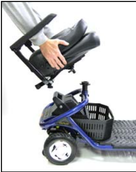
Figure 13. Removing the Seat
