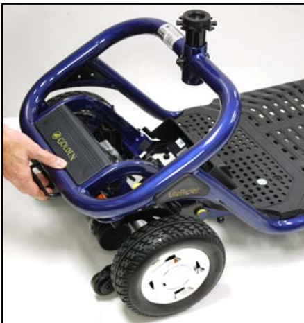
Figure 17. Releasing the Drivetrain
