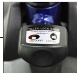
Figure 22. Tiller Raised and Unlocked
