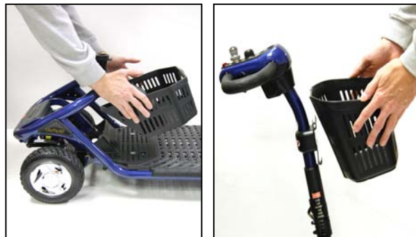
Figure 15. Removing the Baskets
