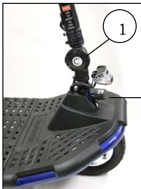
Figure 22. Tiller Raised and Unlocked
