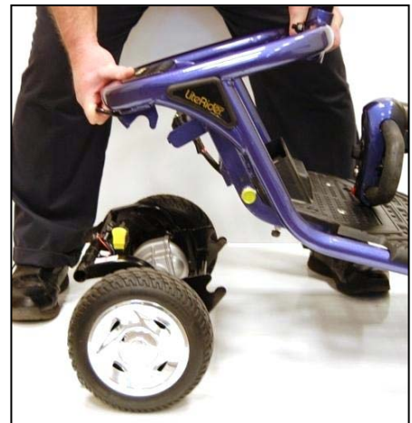
Figure 18. Lifting the Frame
