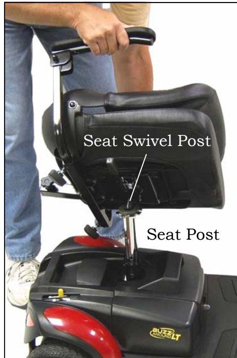
Figure 23. Installing the Seat
