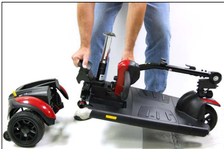
Figure 17. Separating the Drivetrain and Frame
