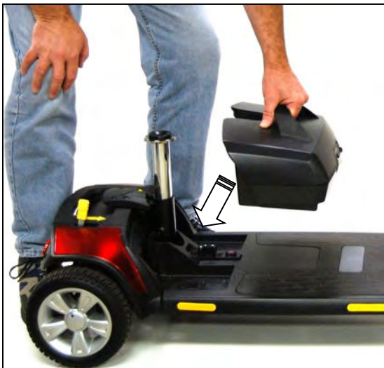
Figure 21. Battery Pack Installation
