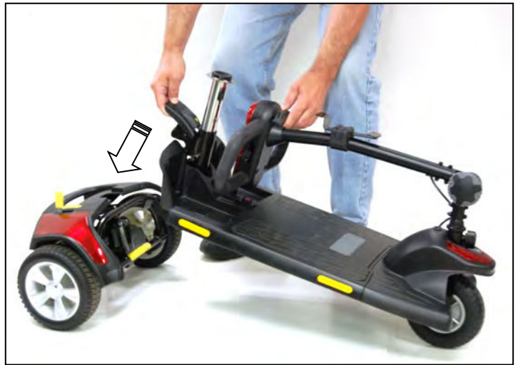
Figure 20. Connecting Frame and Drivetrain
