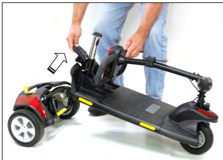
Figure 17. Separating the Drivetrain and Frame
