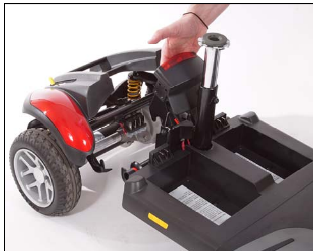
Figure 17. Separating the Drivetrain and Frame
