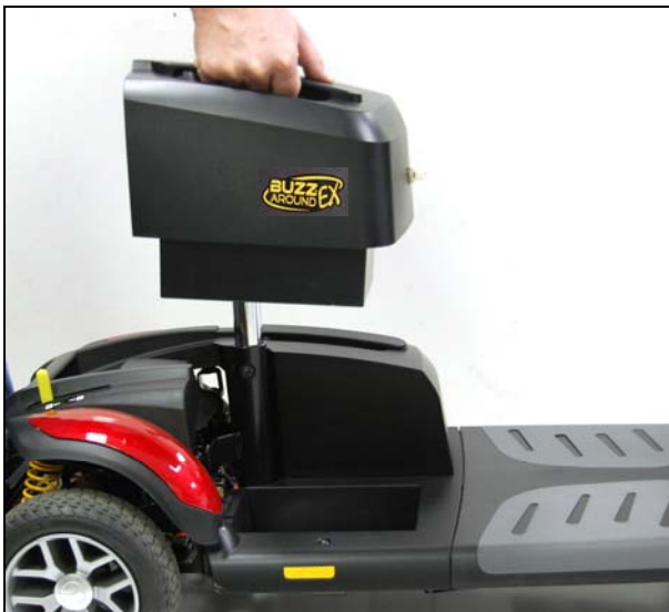
Figure 21. Battery Pack Installation
