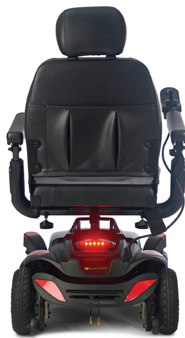
Rear Motion Sensing LED Light
