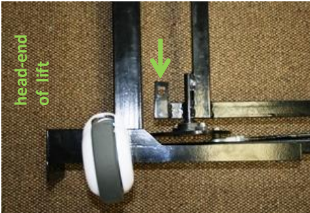
Image 10 – aligning connection for high-low lift
