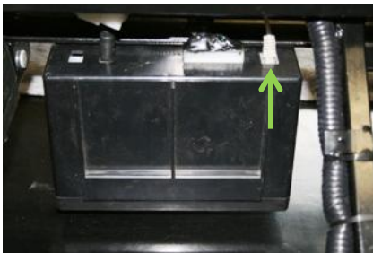
Image 16 – tucking power cord into wire holders
